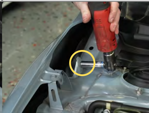
Step 4: Using a 12mm wrench, remove the hood strut ball.
