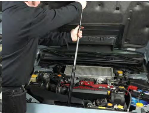
Step 2: Support the hood with a hood prop.
