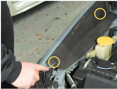
Step 1: Using a small pry tool, remove the push clips from the factory fender cover. Remove the fender cover.
