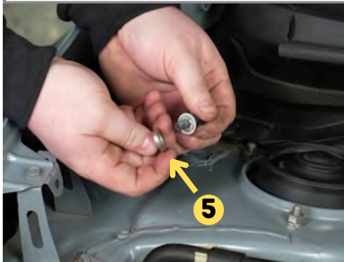
Step 5: Install the provided Strut Spacer onto the hood strut ball, and reinstall.
