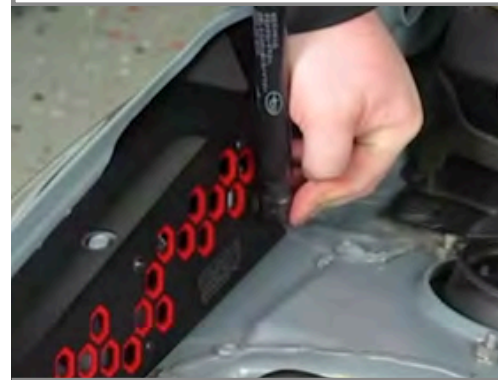
Step 9: Reinstall the hood strut, ensure that the hood strut clip is seated.
