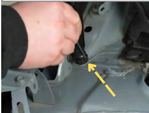
Step 3: Using a pocket screwdriver, pry the hood strut clip up. Remove the hood strut from the ball, and set strut aside.
