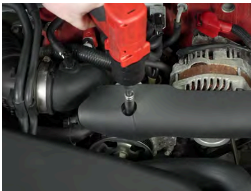
Step 1: Remove the 10mm bolt from the factory alternator cover.
