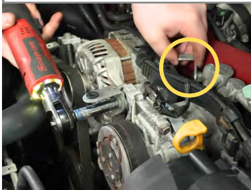
Step 3: Remove 12mm alternator bolt. Hold the nut on the back of the bolt so it does not fall.
