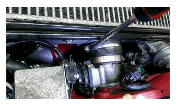
8. Grab the intercooler by the sides and carefully wiggle it out of the engine bay. Be cautious to not hit the A/C line that runs along the fire wall.
