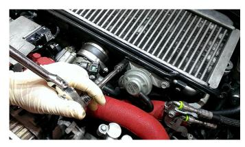
6. Using a flat head screw driver, loosen the hose clamp that is around the turbo discharge silicone coupler.
