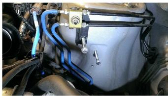
23. Assemble the flat bracket, bolts, washers, spacers and o-rings as shown. Orient the spacer so the side with the groove is facing away from the bracket. The smaller o-ring is used on the 6mm bolt and the larger o-ring is used on the 8mm bolt. Slide the o-ring down into the groove. The o-ring's only purpose is to prevent the spacer from falling off of the bolt during installation or removal. The 02-07 WRX/STI uses the bottom 8mm hole on the bracket as shown.
