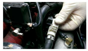
14. Pull PCV fitting from the crank case breather. This is located underneath the turbo on the passenger side of the engine block. The stubby rubber hose might come up with the PCV fitting. This is OK.
