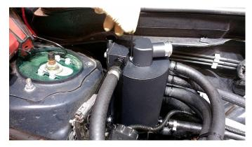
33. Run the 1" hose down the transmission tunnel and secure with the remaining 12" zip ties. Make sure that the hose is not bent or kinked as this will cause operating issues. Keep the hose at least a few inches from your downpipe as you route it down. We do not recommend trimming this hose. The farther back the hose discharges, the less likely you are to smell oil vapor inside the vehicle.
