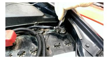
3. Remove the rubber breather hoses from the metal crossover pipe. There are two on the passenger side and one the driver's side. Some vehicles may use spring clamps. You should be able to twist and pull the hoses off once the clamps are removed. If you'd like, you can also remove the metal crossover pipe by removing the 2 bolts that hold it to the intercooler. This is optional. The crossover pipe will not be utilized with the IAG AOS.
