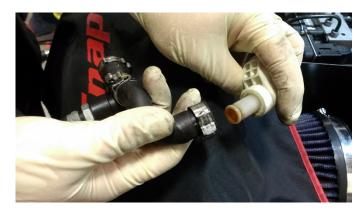
16. Take the ½" rubber cap and place it over the barbed side of the white blow by sensor. Zip tie the cap in place and then plug the sensor back into turbo inlet and reconnect the harness to the sensor.
