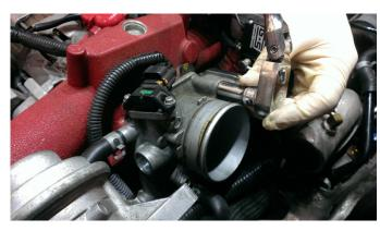
10. Remove the rubber hose from the PCV nipple under the throttle body.
