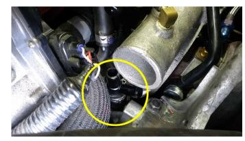
20. For 06-07 vehicles, use a small pick and disconnect the wiring harness from the bracket that is attached to the passenger side strut tower.
