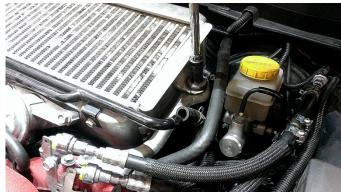
5. Using a 12mm socket, remove the two bolts that hold the blow off valve (BOV) to the intercooler. You can leave the BOV where it sits. Be careful not to lose the gasket.
