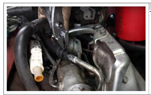
Step 32 pt.2 Tighten new hose clamp
