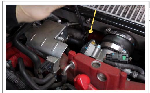
Step 7 pt. 2 Loosen the 8mm hose clamp on the intercooler pipe.
