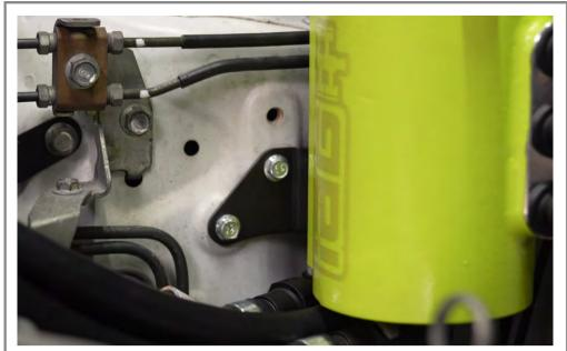
Install the AOS and bracket to the strut tower.
