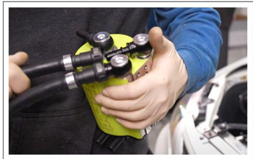
Install the two coolant lines to the AOS.
