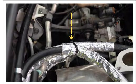
Secure the two hoses together using a zip tie.
