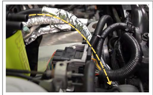
Route hose under coolant hoses and down towards the passenger side valve cover.
