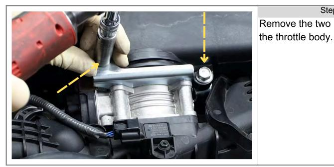
Step 4 Remove the two 12mm bolts on
