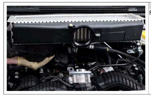
Step 6 Remove the intercooler.
