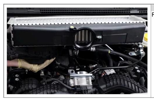
Step 6 Remove the intercooler.
