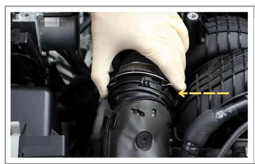
Step 5 Using a pocket screw driver release the charge pipe spring lock.
