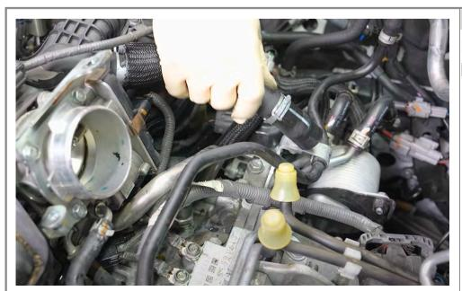
Step 13 pt. 2 Remove the intake manifold hose from the PCV valve.
