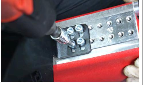
Using a 5mm Allen wrench, Install and tighten the AOS bolts.
