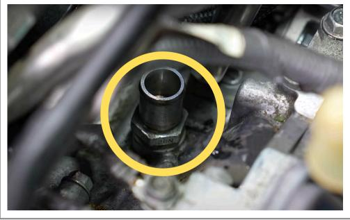
Remove the PCV valve from the block with a 27mm socket.
