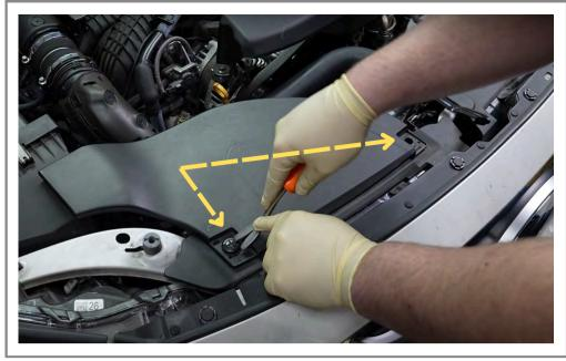
Using a trim pry tool, remove the two clips that hold the air snorkel.
