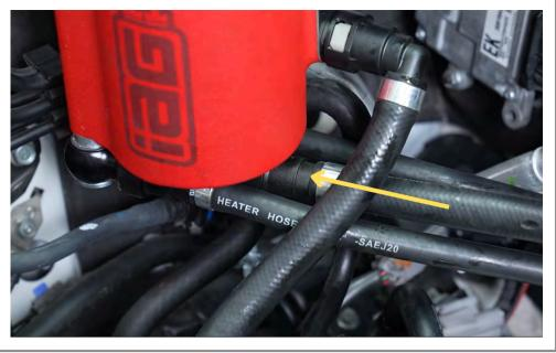
Connect the straight hose end to the bottom drain port of the AOS.
