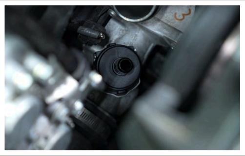
Install the provided Turbo Inlet adapter onto the turbo inlet.
