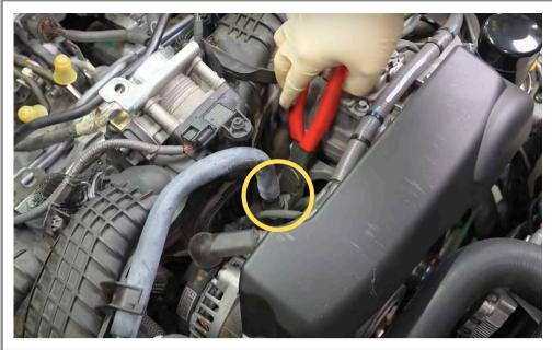
Locate the vent hose in front of the intake manifold.
