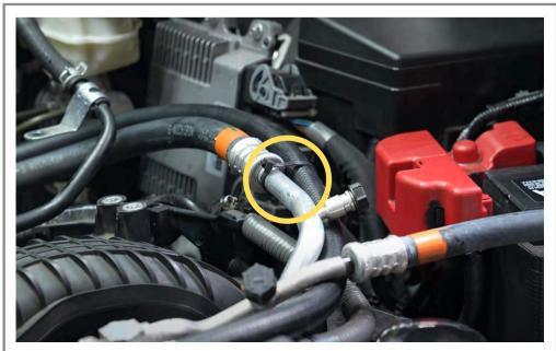
Step 37 pt. 2 Zip-tie the AOS hose to the A/C line as shown.
