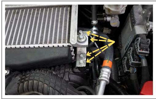
Remove the four 12mm bolts from the intercooler bracket on the passenger side.
