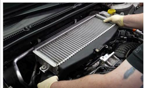
Step 6 Remove the intercooler.
