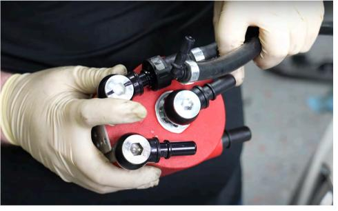
Prepare the 27" AOS Coolant Hose with the 90° end. Install the quick fitting end onto the AOS unit as shown.
