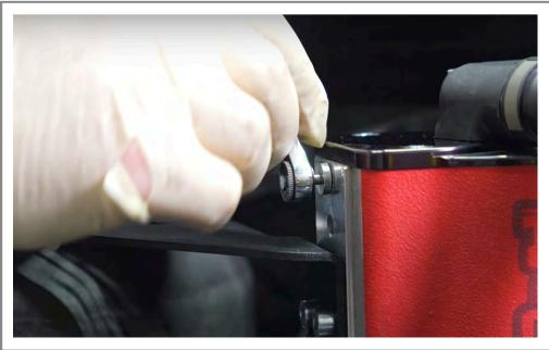
Step 51 Loosen the AOS coolant bleed screw with a 1/8 Allen wrench.
