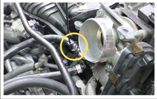
Zip-tie the AOS coolant hoses together next to the throttle body.
