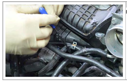
Step 28 Remove the pinch off pliers.
